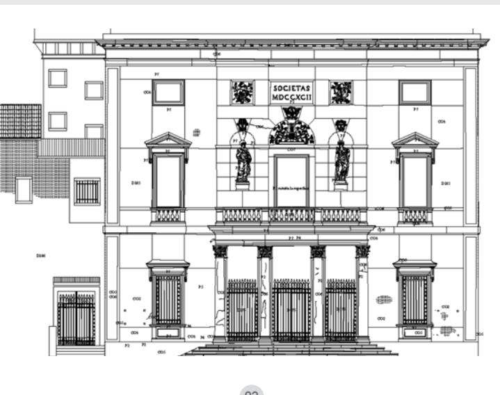
Fig 4. Detailed drawing with single marble slabs related to a fixed price contract with detailed descriptions of complete restoration works
